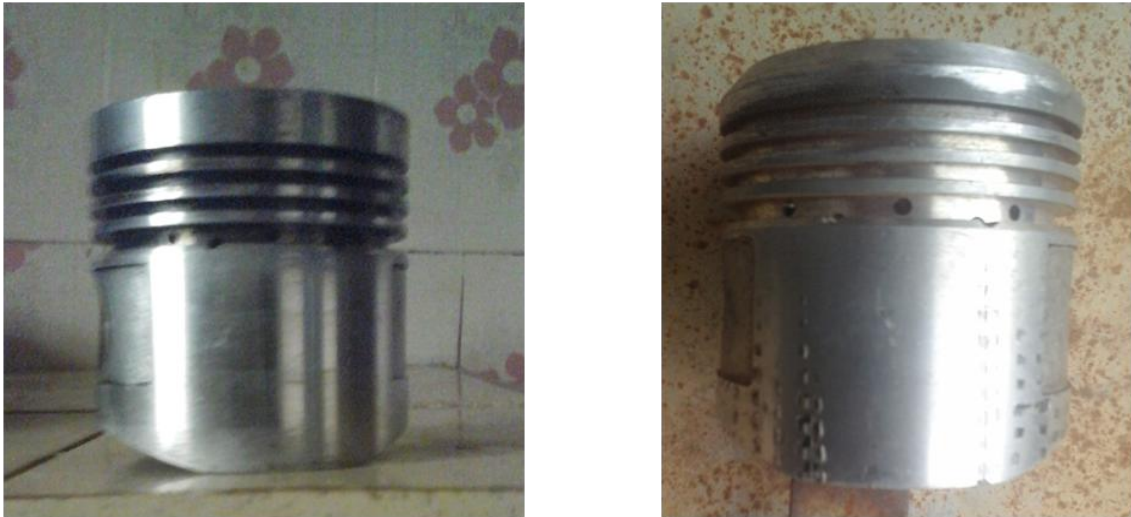
Fig. 3 Piston crown modification
