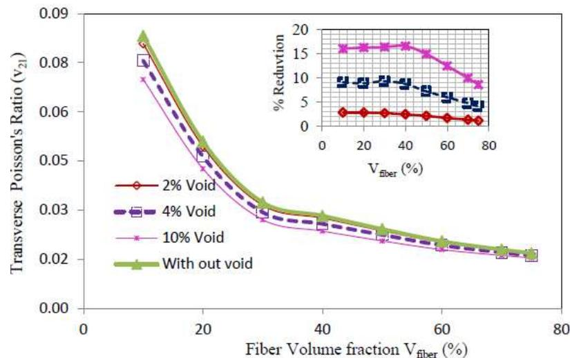
Fig.19.  $v_{21}$  of T-300 reinforced composites with void at 2% fullerene volume fraction
