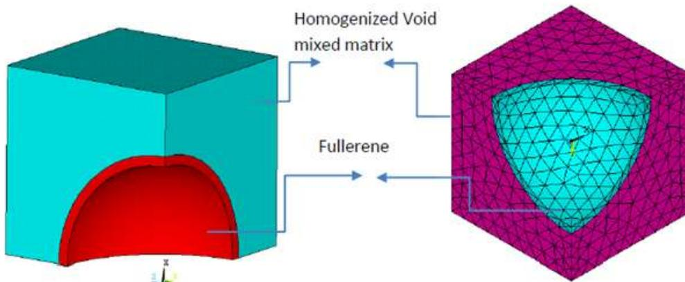
Fig. 10. a Finite element model at 10% Vp
