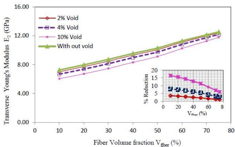
Fig.18 E<sub>2</sub> of T-300 hybrid composite with void at 2% fullerene volume fraction
