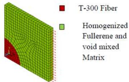
**Fig.15. b. Fe Model under Transverse Loading at 10%  $V_{\text{fiber}}$**
