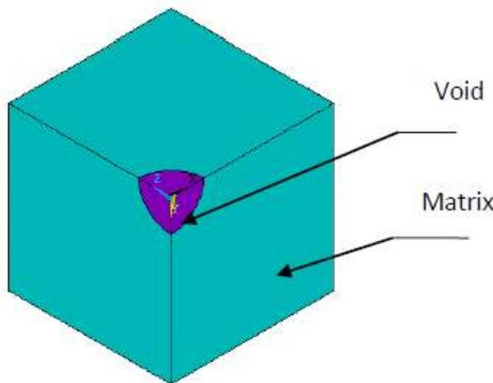
Fig. 3.a Geometrical model with void at 2% Vv
