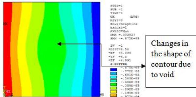
FIG. 5.B UX- CONTOUR WITH VOID
