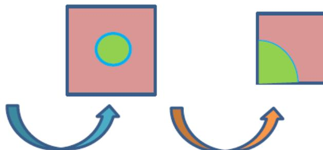
Fig.14.b isolated Unit cell and one eighth in homogenized fullerene and void mixed matrix portion of unit cell
