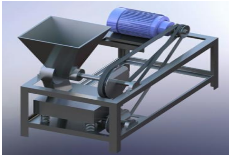
Figure 1: Isometric Model View of Dried Cassava Pellets Grinding Machine
