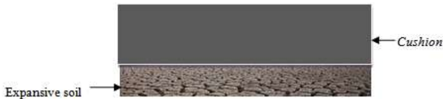
Fig. 4 Sub Excavating or Replacing the Expansive Soil by Cushions
