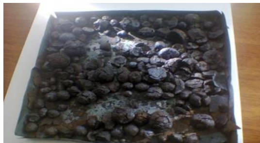
Fig. 3. Granules produced using water after heating
