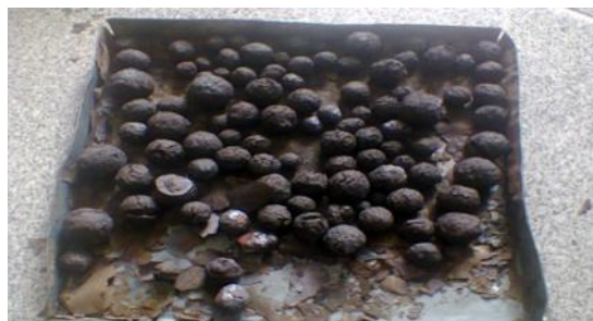
Fig. 4. Granules produced using the specially formulated binder after heating
