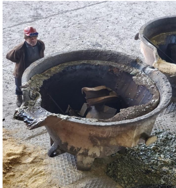
Figure 1. Placement of steel scrap in the ladle
