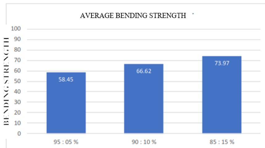
Figure 4. Average Bending strength for each weight fraction
