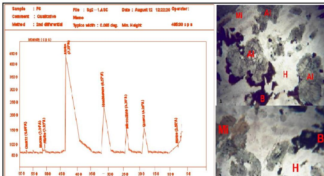
Fig. 2: XRD traces and Syenite mineral slides (A-albite, B-biotite, M-microcline, H-hornblende)
