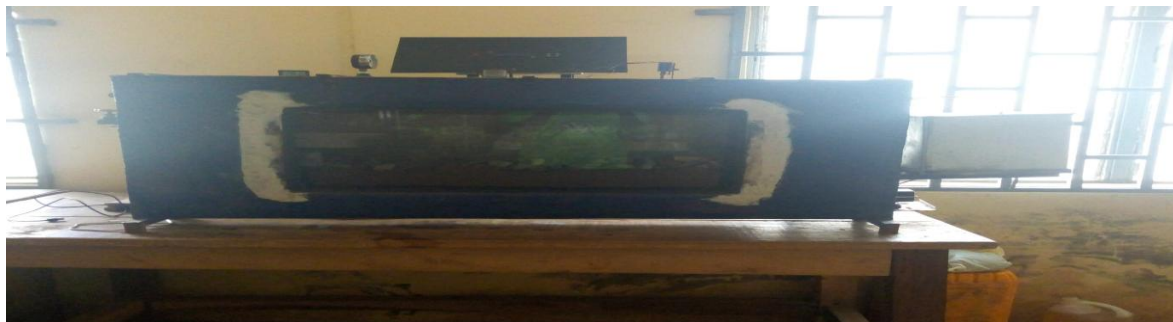
Plate 2.0: Test chamber (Sand box) and condenser
