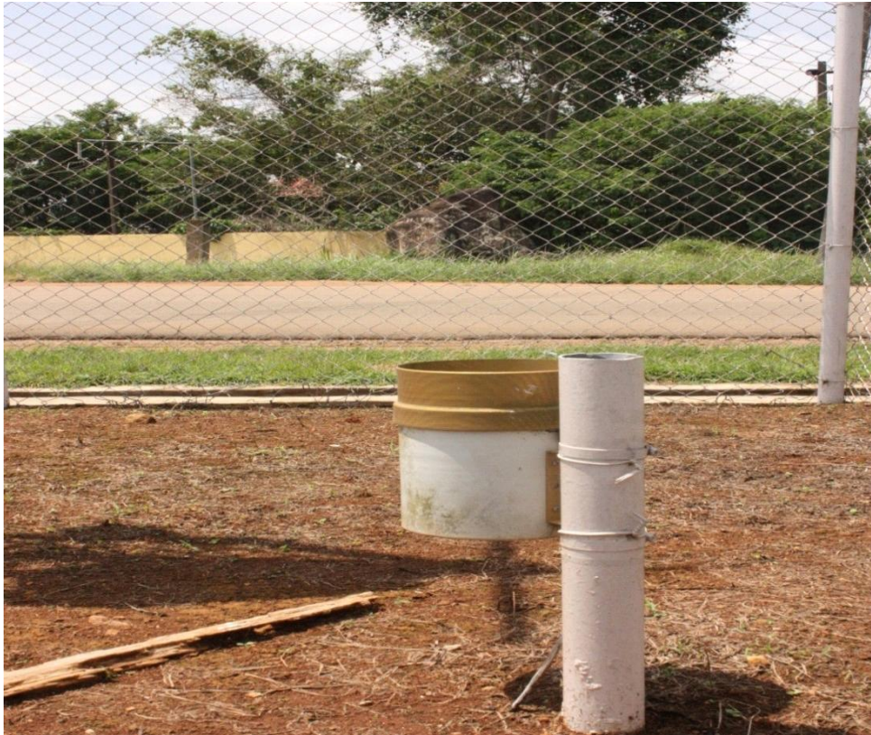
Figure 3.3: The TRODAN observatory garden at FUTA uses a tipping bucket rain gauge.
