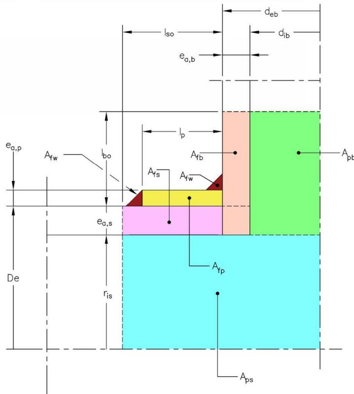
**Figure 1: Illustration of set-in flush nozzle with reinforcing plate on a cylindrical shell**
