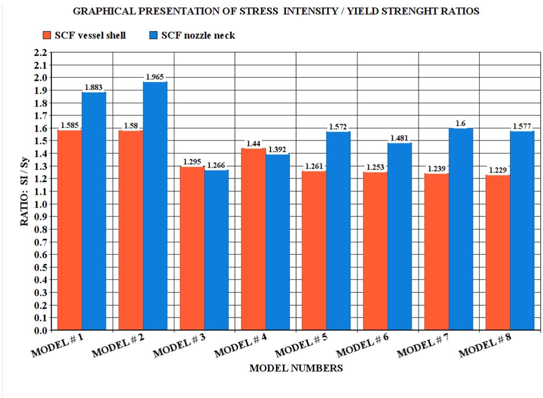
Figure 6: Graphical presentation of stress intensity / yield strength ratios
