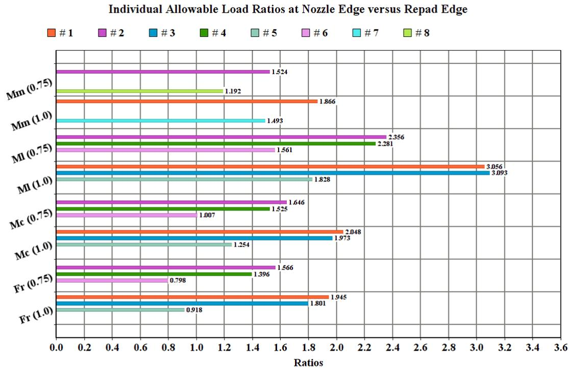
**Figure 7: Individual allowable load ratios at nozzle edge versus repad edge**
