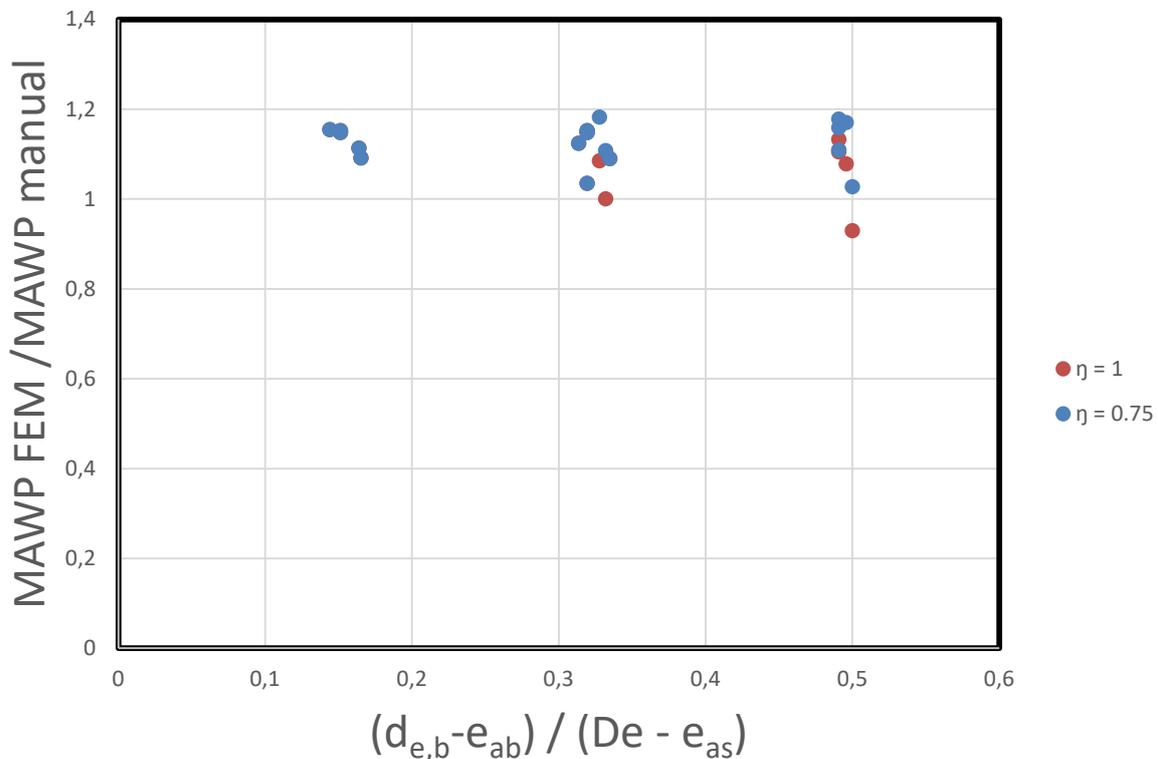
Figure 10: Comparison FEA results versus manual calculations
