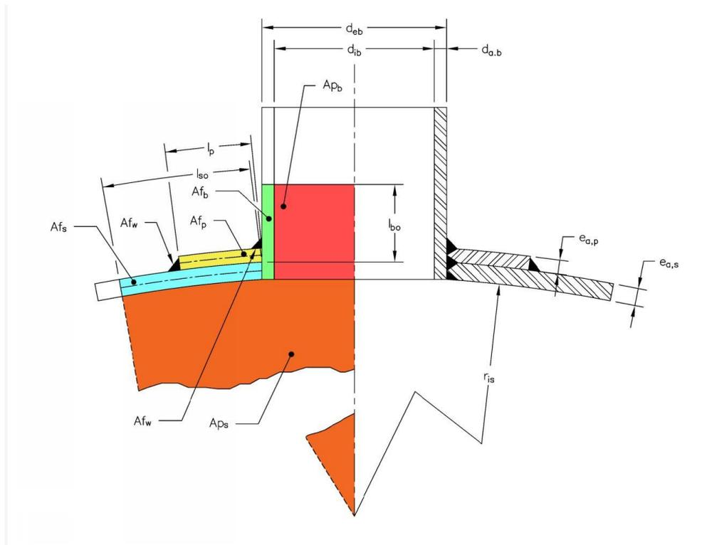
Figure 2: Illustration of set-in flush nozzle on spherical shell with reinforcing plate
