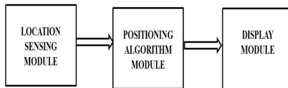
Figure 1.1: A functional block of an Indoor Positioning System
