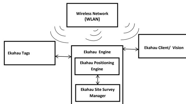
Figure 3.1: The Block Diagram of Ekahau RTLS System [19]
