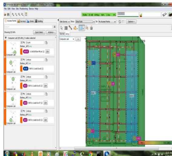
Figure 4.2: Data rate – Computer Laboratory
