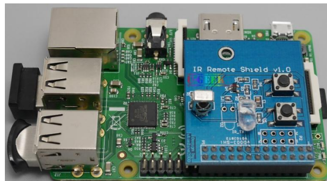
Figure 5. Pairing Raspberry and infrared transceiver module for TV control
