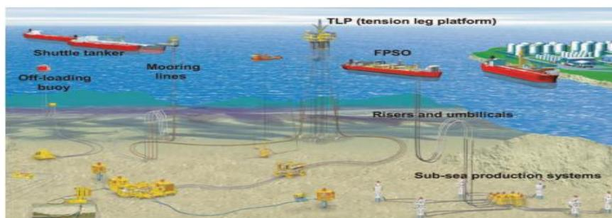
Figure 2 - Offshore production systems
