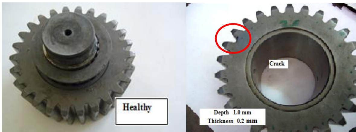
Fig. 4 Wind turbine planetary gearbox healthy components and gear tooth crack
