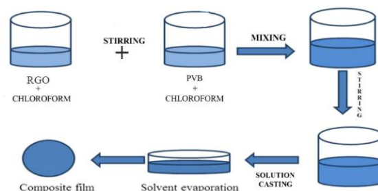
Figure-1 Fabrication process of PVB-RGO composite films
