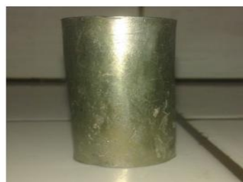
b) Cylindrical mould of Diameter = 15 mm; Height = 40 mm
