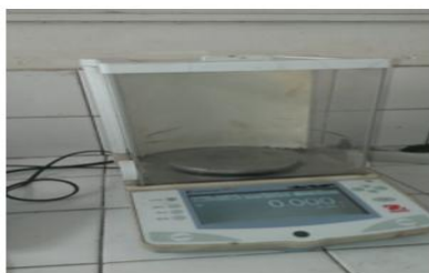
a) Balance with precision Explore-pro (0-210g, with E = 0.0001g)
