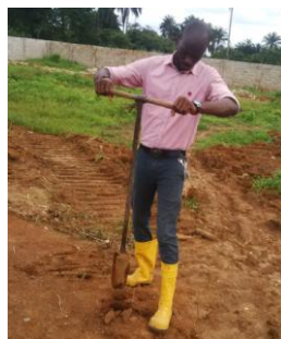
Plate 1. Sampling using Hand Auger Plate 2. Samples bagged and labeled
