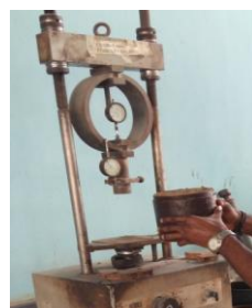
Plate 6. CBR testing of soil sample
