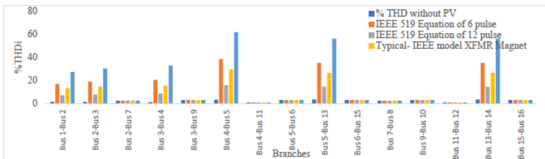
Fig.13. THDi without and with PV connection with different types of converter harmonic models
