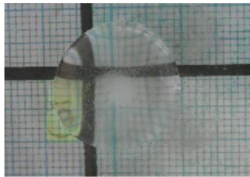
(f) Propagation of the vortex towards the drop sides of the right half, continuous increase in the drop height at the T.E.
