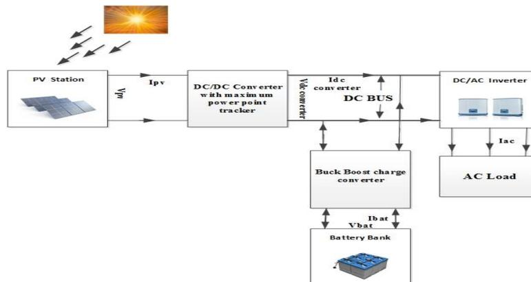
Fig. 4. Block diagram of Stand-alone photovoltaic System
