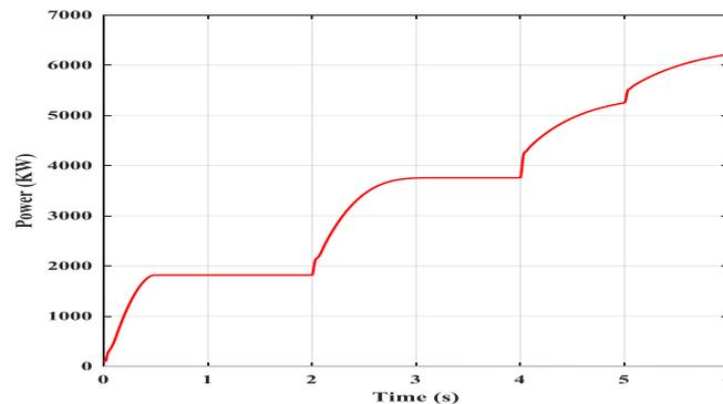
**Fig. 8. Variation of PV power station due to variation of irradiation with time**
