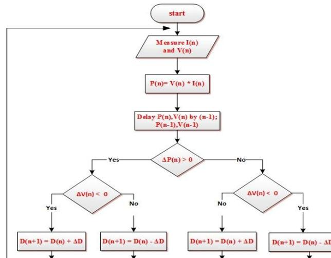
Fig. 5. Flowchart of the Perturb and Observe method
