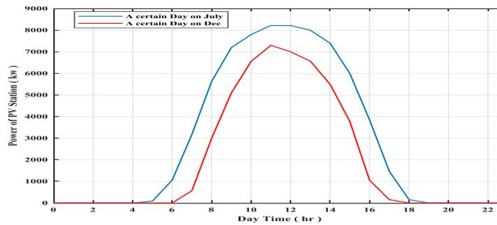
Fig. 12. Power produced from photovoltaic power plant during one day
