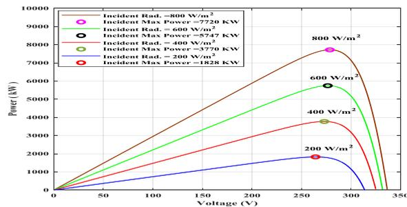
(b). Power vs. Voltage for the designed standalone solar station
