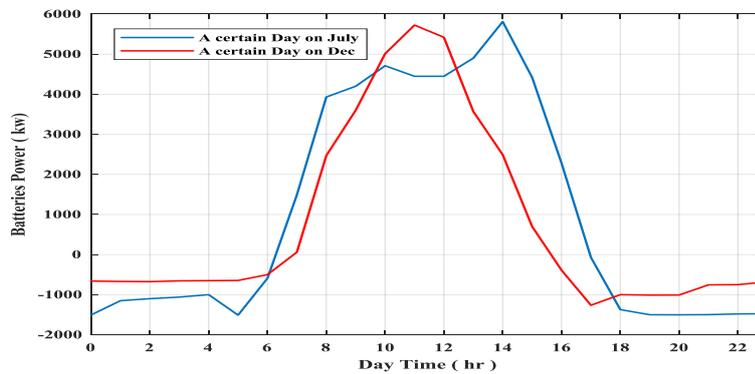
Fig. 13. Transferred power from or to the batteries during the day
