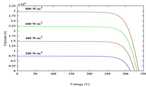
(a). Current vs. Voltage for the designed standalone solar station
