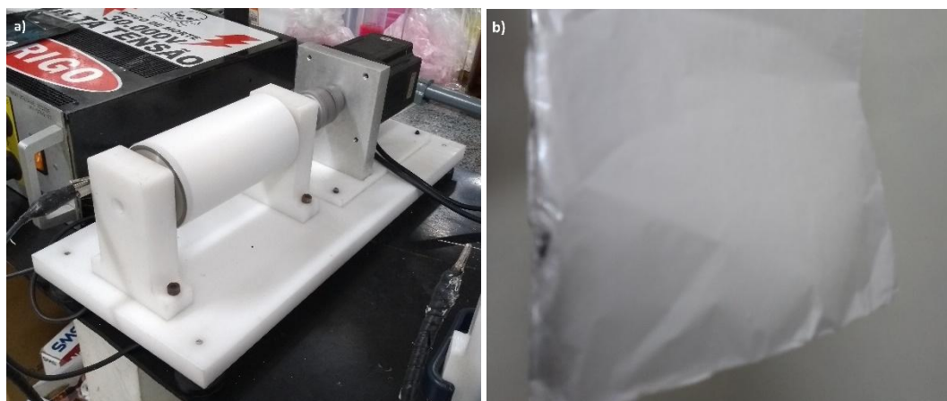
Fig. 3. Electrospun PCL fibers and collected by the rotating cylinder device (a) and fibrous PCL mat removed after its production (b).
