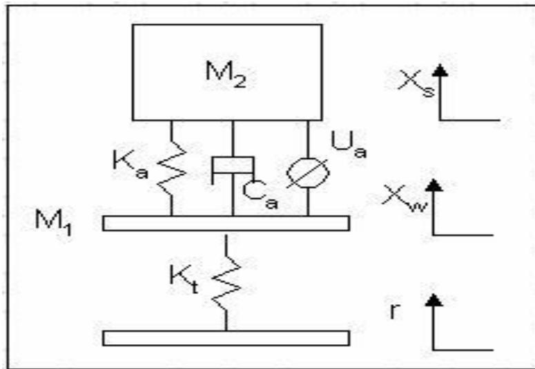
Figure 3: Active Suspension for Quarter Car Model
