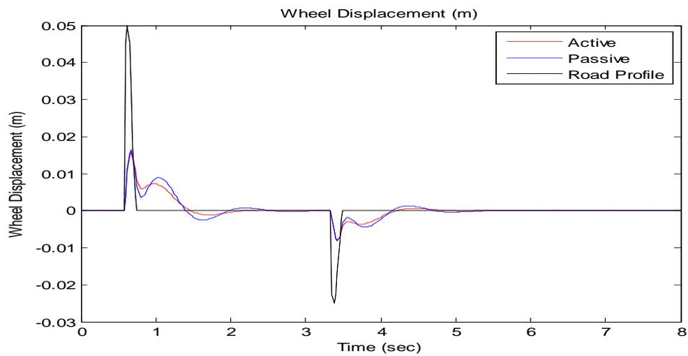
Figure 14: Wheel Displacement with Road Profile 2
