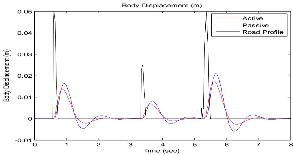
Figure 7: Body displacement with road profile 1
