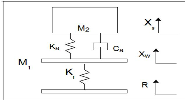
Figure 2: Passive Suspension for Quarter Car Mode
