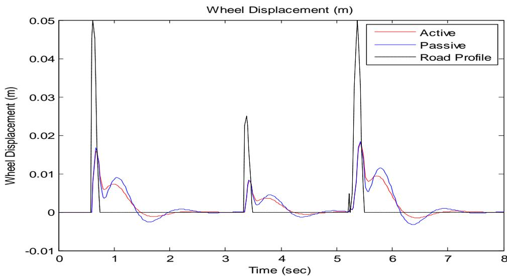
Figure 9: Wheel Displacement with road profile 1
