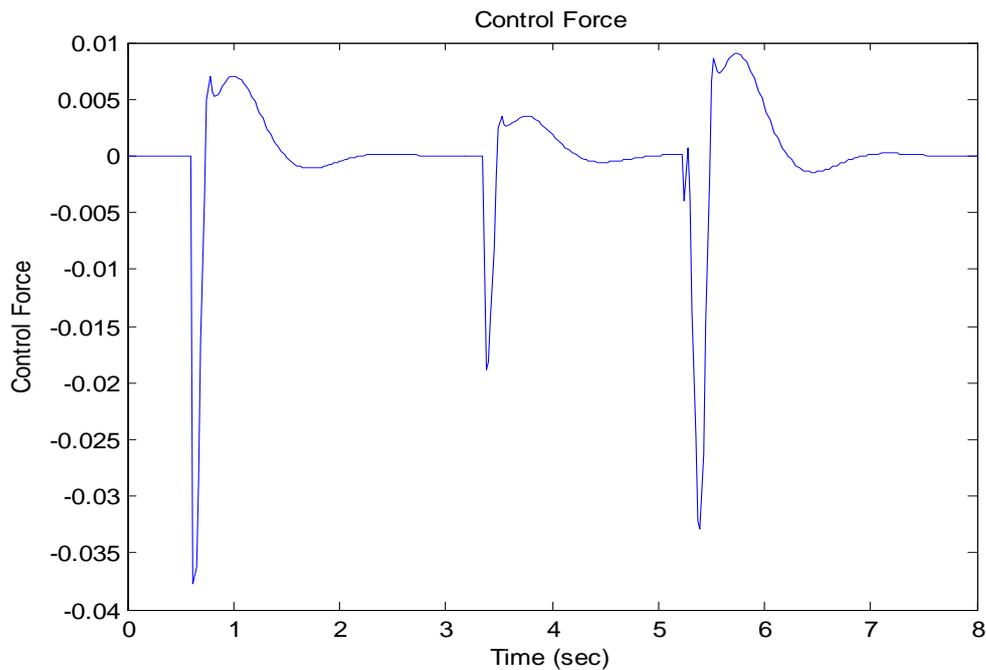
Figure 6: Force generated using LQR Controller with road profile 1
