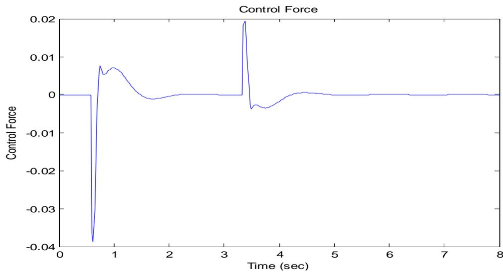
Figure 11: Force generated using LQR Controller with road profile 2
