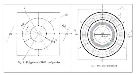
The resultant AM arbitrarily positioned in the plane P can be treated as a composite gyro having similar properties as the dual DC motor model [1]. That means if any torque applied to the platform P the system will react as per well-known gyro properties. The said torque can be arbitrarily positioned in the space having two components i.e. in the plane P and perpendicular over it. Both components will generate adequate reaction of the AM.
