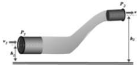
Figure 3. Flow of Fluid Using Pressure
