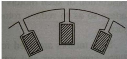
Figure 3.1.3-6: Class E rotor conducting bars arrangement
