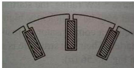
Figure 3.1.3-3: Class B rotor conducting bars arrangement
