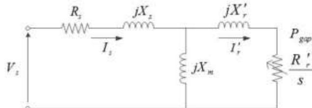
Figure 3.1.4-1: Steinmetz equivalent circuit machines.
