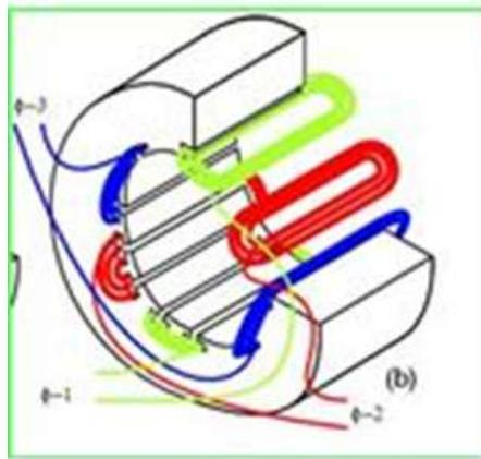
Figure 3.1.2-1: 3 phase stator winding layout
