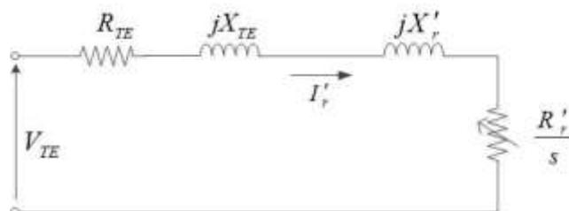
Figure 3.1.4-3: Thevenin equivalent circuit.
