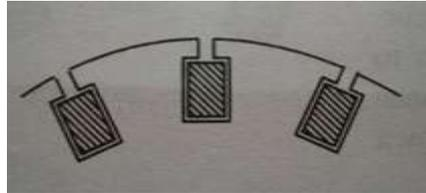
Figure 3.1.3-2: Class A rotor conducting bars arrangement
