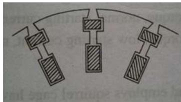
Figure 3.1.3-4: Class C rotor conducting bars arrangement
