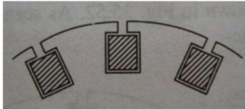
Figure 3.1.3-7: Class F rotor conducting bars arrangement
