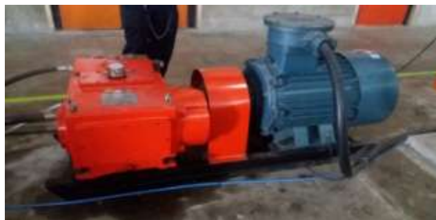
Fig. 2. Recrocating pump: main component of hydraulic powerpack
