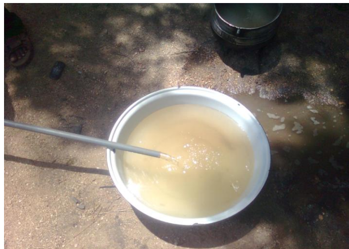
Pump testing at Varam @ 6Litres per minute
