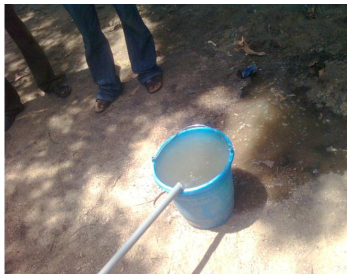
Pump testing at Varam @ 6Litres per minute
