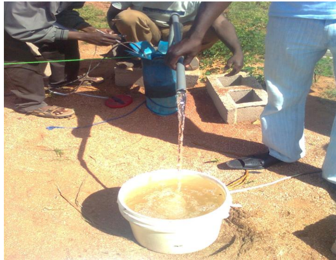
Pump testing at Bogot @ 4Litres per Minute
