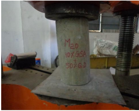
Fig.7 Specimen for compressive strength of cylinder
