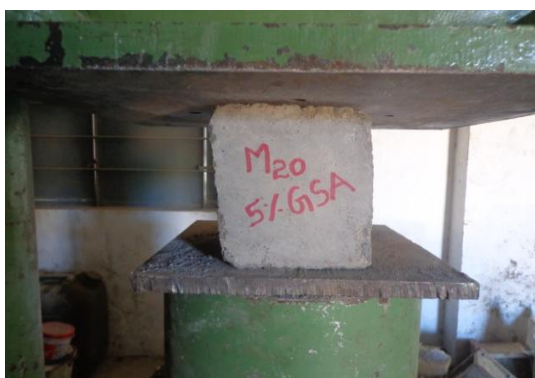
Fig.4 Specimen for Compressive Strength of Cubes
