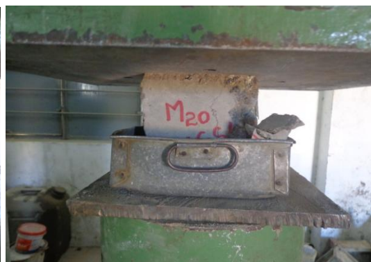
Fig.5 Failure of compressive cube
