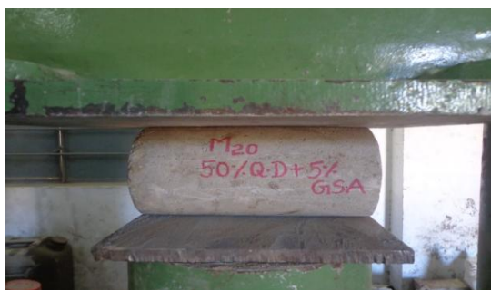
Fig.10 specimen for split tensile strength of cylinder
