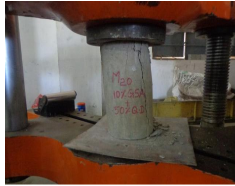
Fig.8 Failure of compressive cylinder
