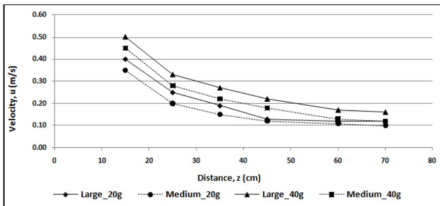
Figure 8: variation of sand frontal velocity with different nozzles (20g and 40g)
