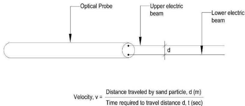
**Figure 2:** velocity measurement of sand particle using electric probe
