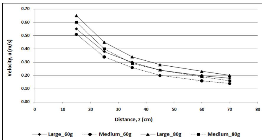
Figure 9: variation of sand frontal velocity with different nozzles (60g and 80g)
