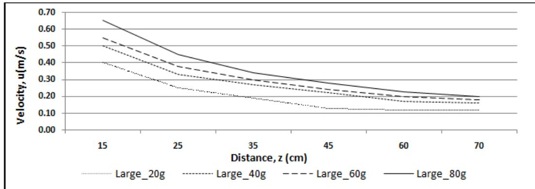
**Figure 5:** variation of sand frontal velocity with different masses for large nozzle
