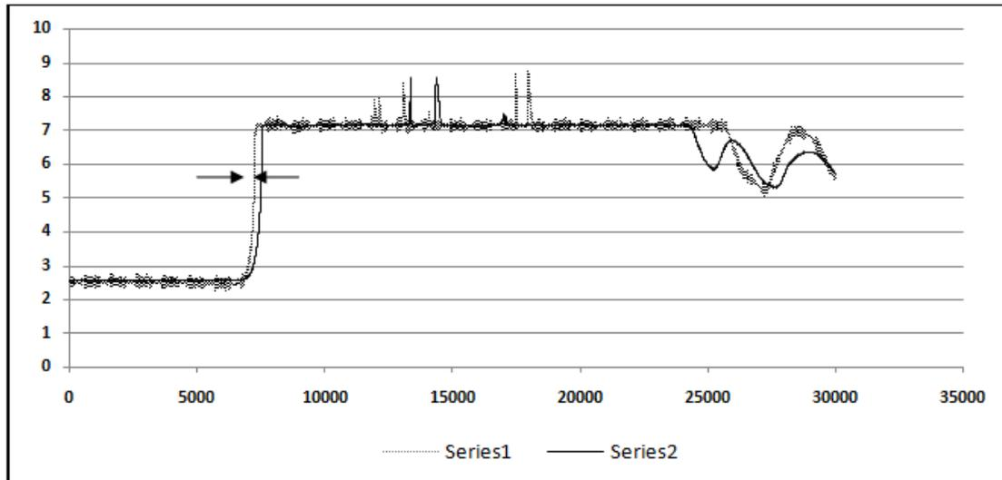
**Figure 3:** voltage signal for sand mass 40g and large nozzle at position 15 cm.
