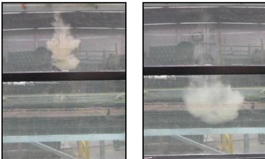
**Figure 6:** 80g sand mass released from large nozzle and pictures taken at 3 and 7 seconds from the time of releasing
