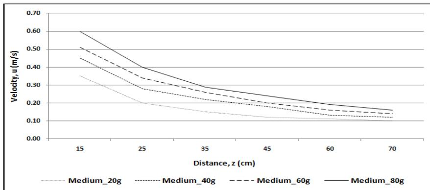
Figure 7: variation of sand frontal velocity with different masses for medium nozzle
