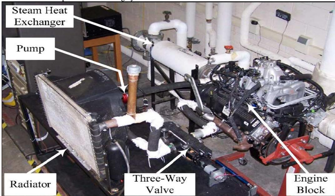
Figure 5.2 Experimental scale cooling control system hardware for real-time algorithm studies
