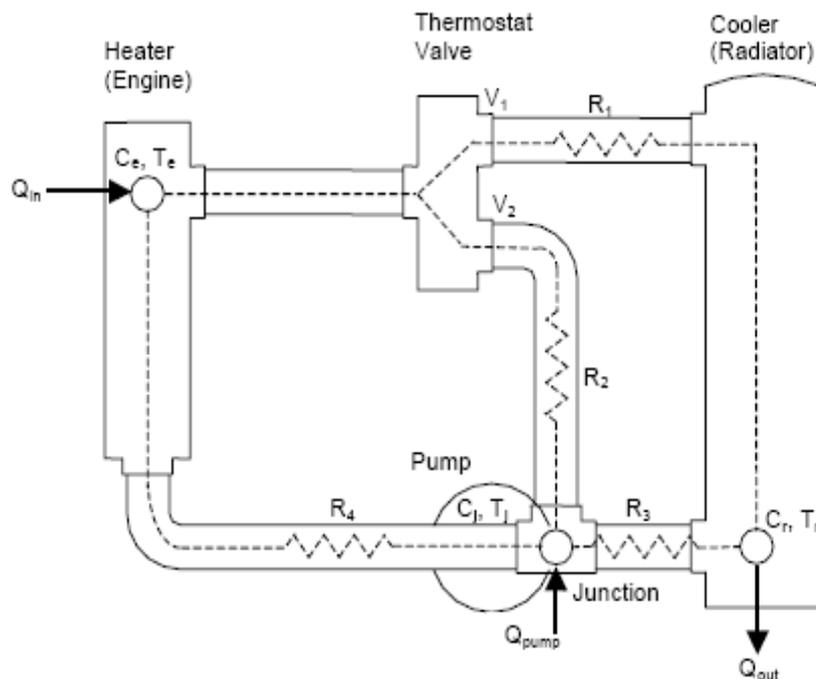
Figure 5.3: Experimental cooling system with flow direction
