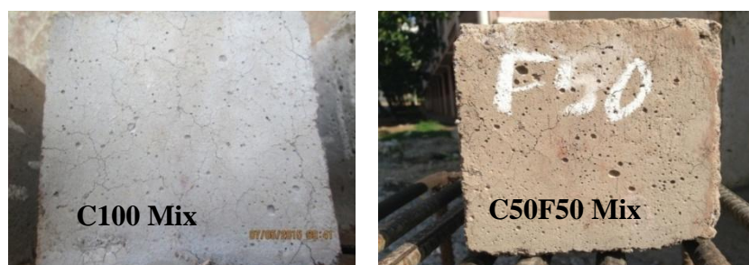
Figure 1: Colour Change at 800°C
