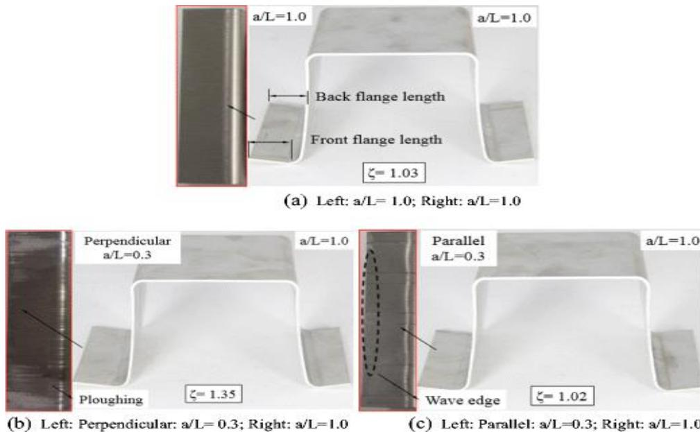
Fig. 4 Texture orientation effect on the draw-ability and part quality with a blank-holding force 10 kN for cold stamping processes
