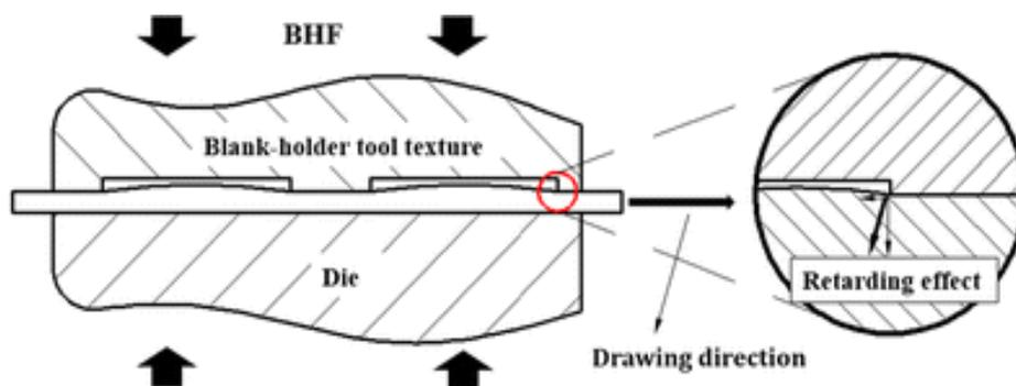
Fig. 5 Illustration of the ploughing effect on the material drawing using the perpendicular tool texture
