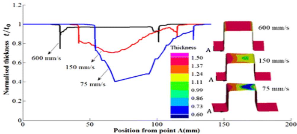
The work described in this paper has investigated the effect of rectilinear macro-textures on metal flow in the cold and hot stamping of a top-hat shape; a channel with flanges. Perpendicular tool textures corresponding to the material flow direction had constraint effect on material flow as the material deformation due to the large blank-holding force, the flange ratio was increased to 1.35, compared with 1.03 using non-texture on the two sides in cold stamping process.
