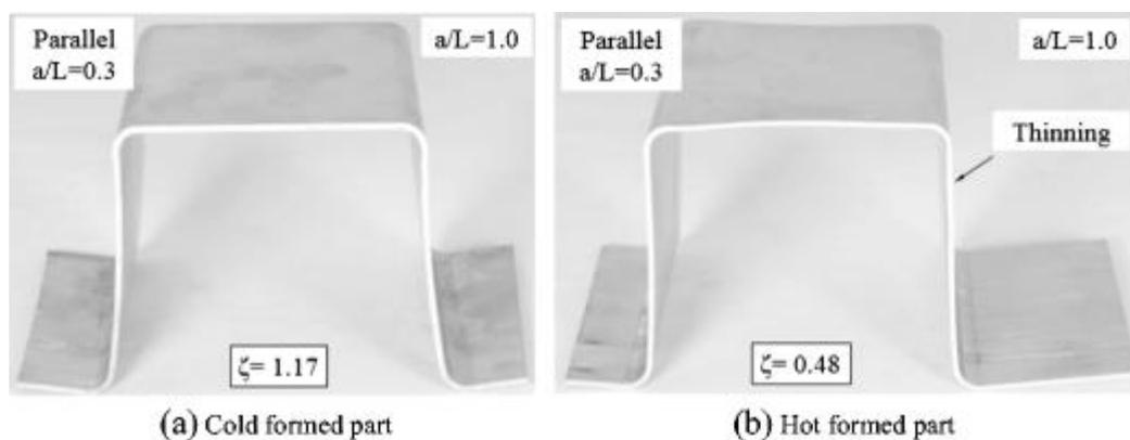
**Fig. 6** Effect of tool texture design on the draw-ability in the stamping processes. The tool texture designs are: *Left*: Parallel  $a/L = 0.3$ ; *Right*:  $a/L = 1.0$  with blank-holding forces **a** 30 kN and **b** 15 kN
