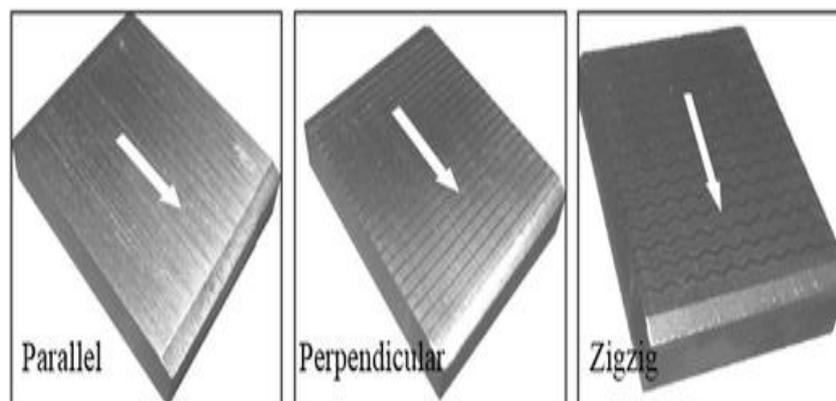
Commercial AA6082-T6 condition aluminium sheets with a thickness 1.5 mm were used as test-pieces. The chemical composition is provided by the materials supplier and given in Table 1. The typical solution heat treatment temperature for the alloy is 525 °C.
