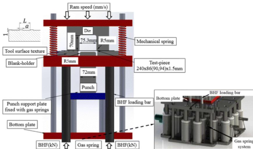
(b) Schematic design of the stamping rig
