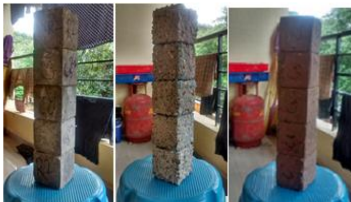
Fig 5: Specimens exposed to ordinary water, sulfuric acid (5%) and hydrochloric acid (5%)
