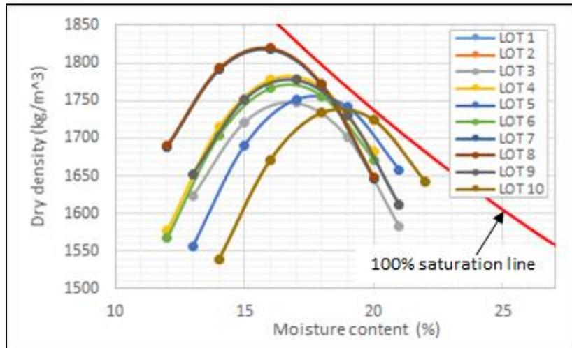
**Figure 7:** Compaction curves derived from the Standard Proctor test of the different soil samples. All curves are reasonably constrained by the 100% saturation line.
