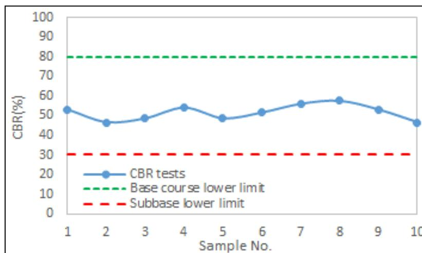
**Figure 8:** Results of CBR test for the soil samples under consideration. The minimum limit ( $\geq 30\%$ ) for soaked subbase is the dashed red line while the dashed green line is the minimum limit ( $\geq 80\%$ ) for dry base course.
