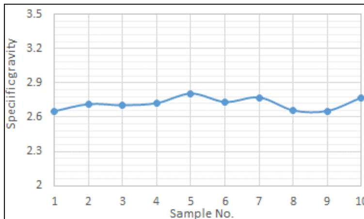
Figure 6: Plot of specific gravity of the tested soil samples. This is broadly within the range of known specific gravity for soils.
