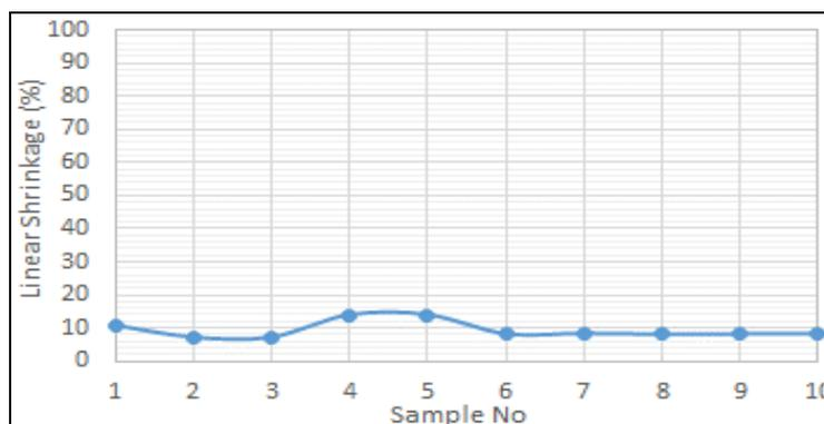
Figure 4: Percentage linear shrinkage determined for the soil samples. All the samples (except 1, 4 and 5) are below the maximum recommended limit of 10% for sub-grade and sub-base soils.
