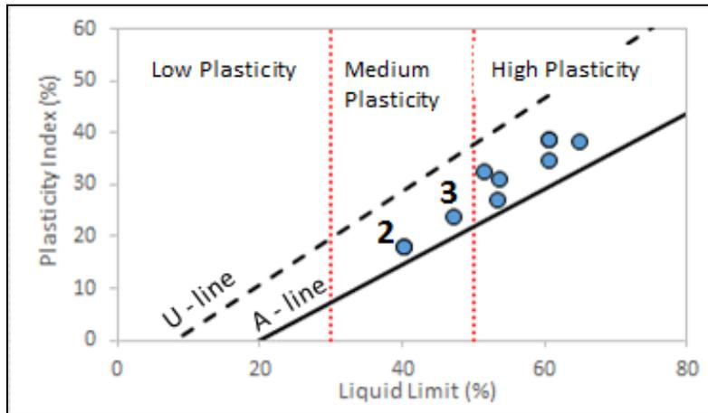
Figure 5: Plot of Atterberg Limits tests results on the Casagrande Plasticity Chart. Samples grade from medium plasticity (samples 2 and 3) to high plasticity.
