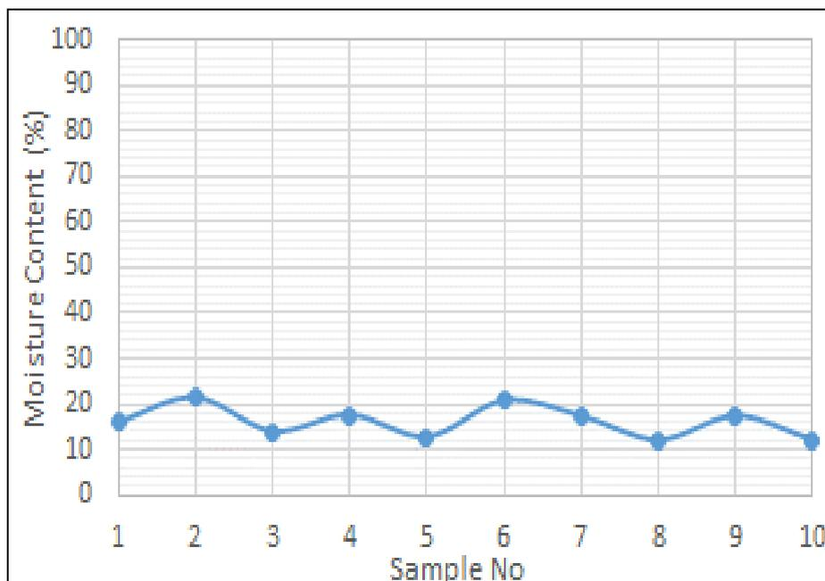
Figure 2: Plot of the average moisture content for each of the soil samples shows variation between 12 % and 21.3 %.
