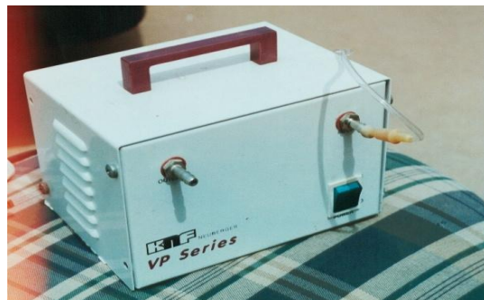
Plate II: Pictorial view of the Vacuum Pump (VP1 PUMP)
