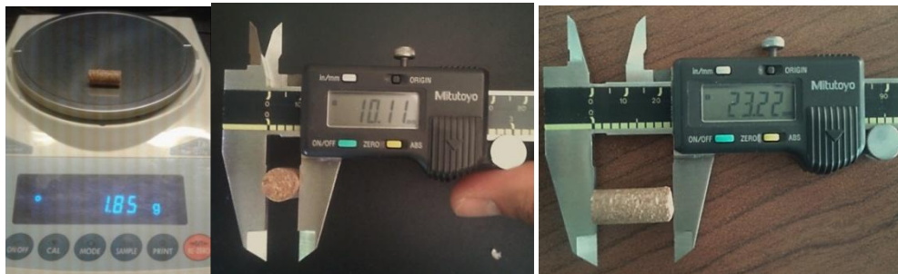
Fig 2 Equipment and procedure followed to determine unit density.
