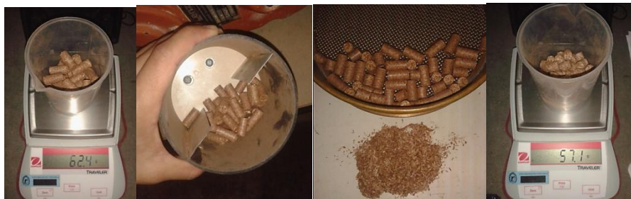
Fig.4. Equipment and procedure followed to determine durability.
