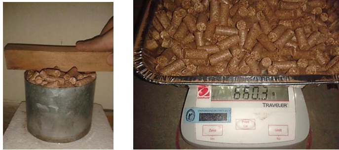
Fig.3. Equipment and procedure followed to determine bulk density.
