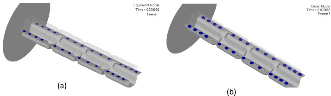
Fig 3 Model setup (a) Equivalent model and (b) Detail FE model
