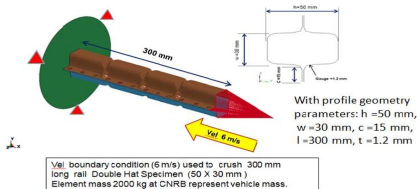
**Fig 2** Crash simulation of a spot-welding beam against a rigid wall
