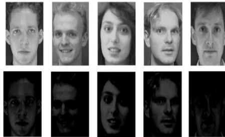
Fig 11: Decrease the Brightness by Subtracting 140 from Each Pixel.
