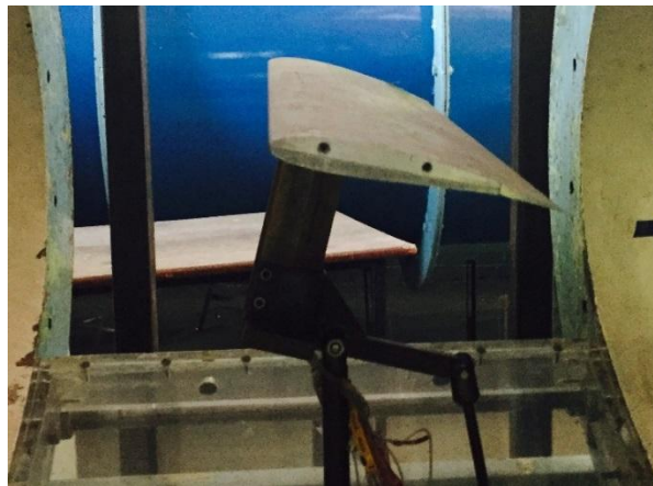
Figure 9, airfoil section in wind tunnel.
