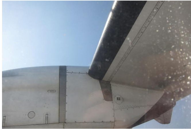
Figure 4, rubber leading edge for ice removal.
