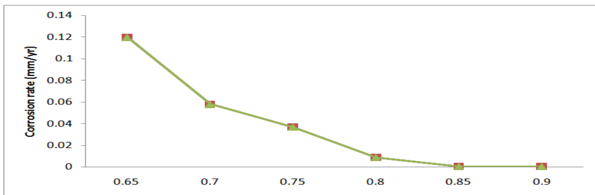
Fig. 9: Effect of variation in polarized potential of specimen on specimen corrosion rate
