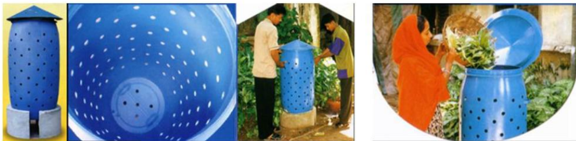
Fig. 5: Construction, installation and use of barrel composting developed by waste concern (Concern, 2005b)
