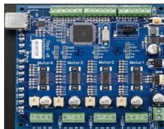
Figure 5: TinyG CNC controller board [12]
