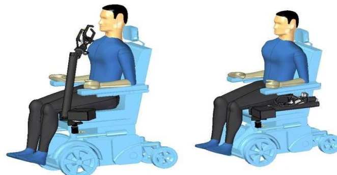
Figure 1: The general layout of the WMRA in extended and folded position
