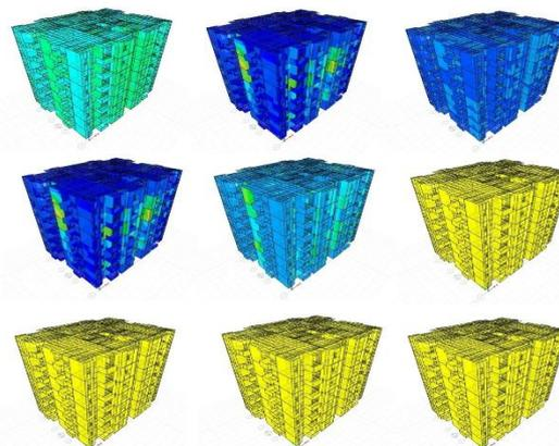
Figure 4: Shell stresses: model 1; load combination 5
