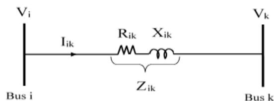
Figure 2: Transmission line model of a power system network
