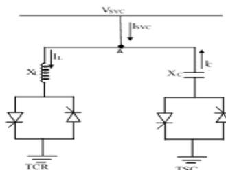
**Figure1:** Functional diagram of a TCR-TSC SVC
