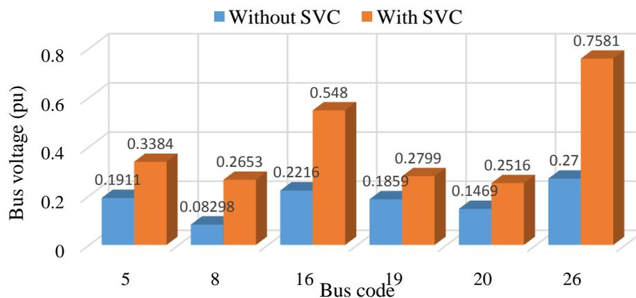
Figure 4: Weak bus voltage compensation representation
