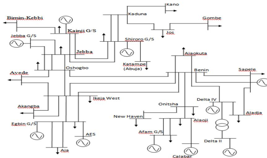
Figure 3: The 330kV, 28-bus Nigerian power system (National Control Centre, Power Holding Company of Nigeria, 2012)
