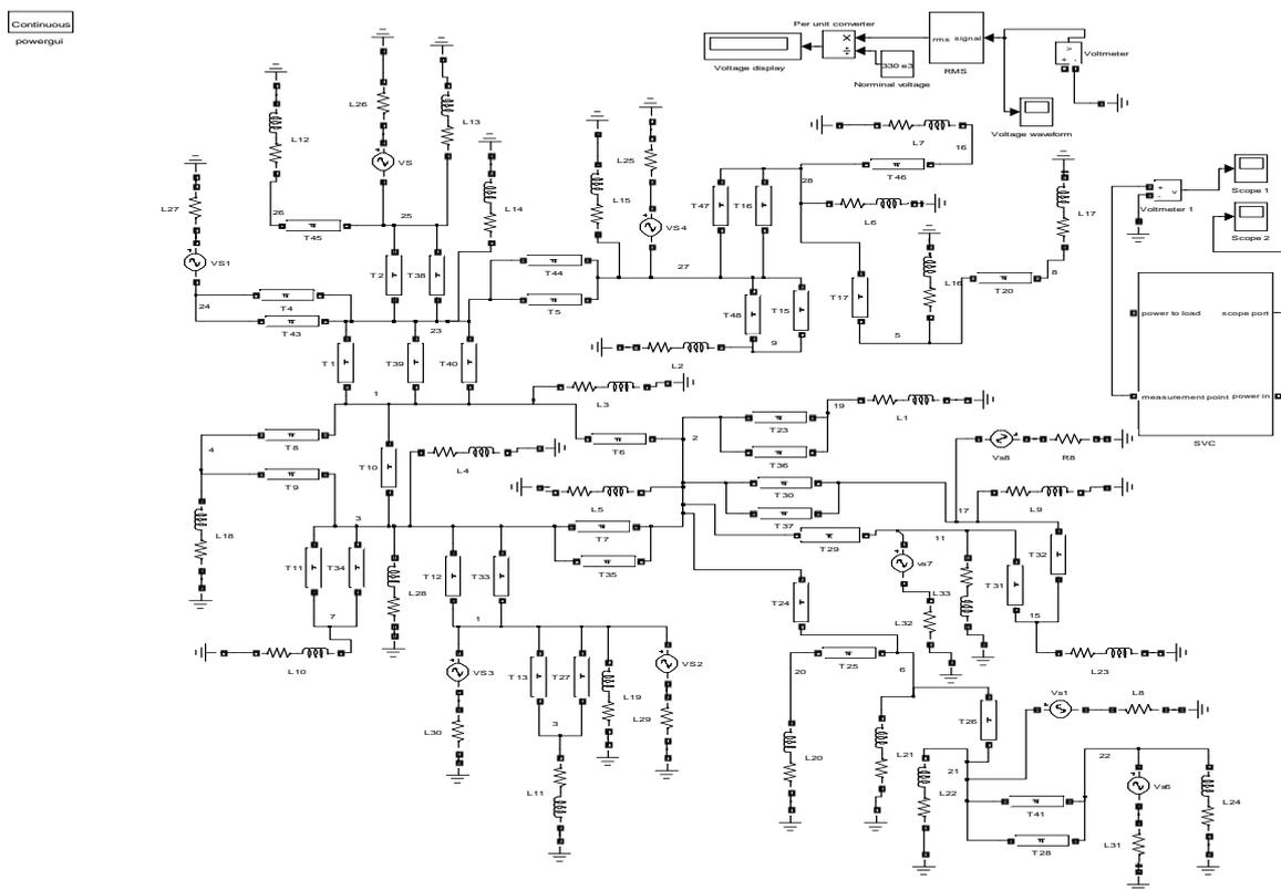
Figure 4: SIMULINK model of the Nigeria 330kV, 28-bus power system
