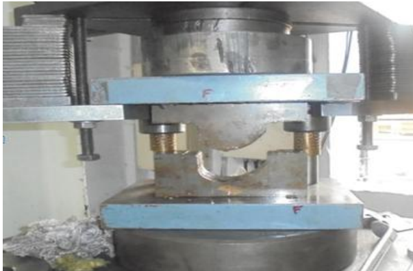
figure 7:Die Fixed in hydraulic press
