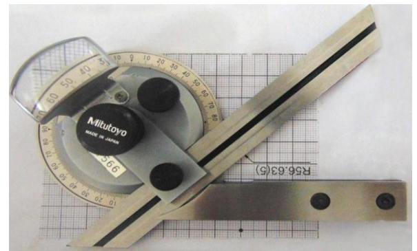
figure 10-Measurement of spring back using bevel protractor
