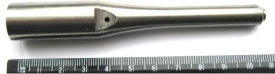
e) rod working tool with the central channel
