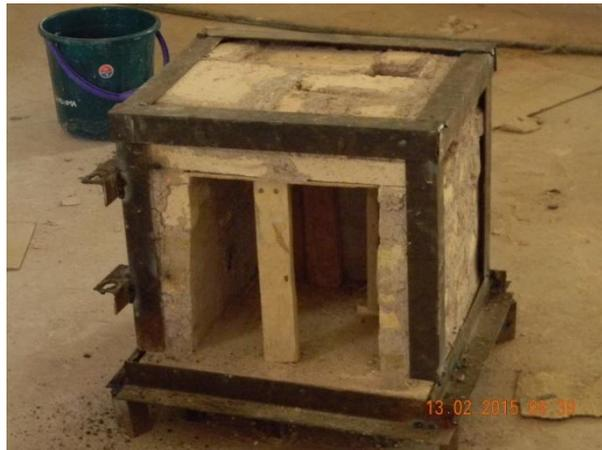
**FULLY CONSTRUCTED PROTOTYPE GAS FIRED KILN**
