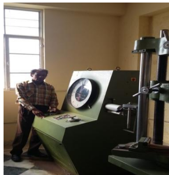
Figure- Universal Testing Machine with Plotter & Hydraulic Load Dial
