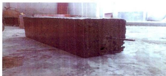
FIGURE:- Beam with sulphur coated steel bar
