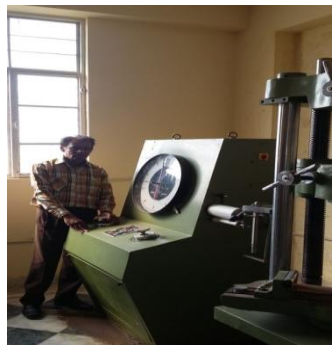
Figure- Universal Testing Machine with Plotter &amp; Hydraulic Load Dial
